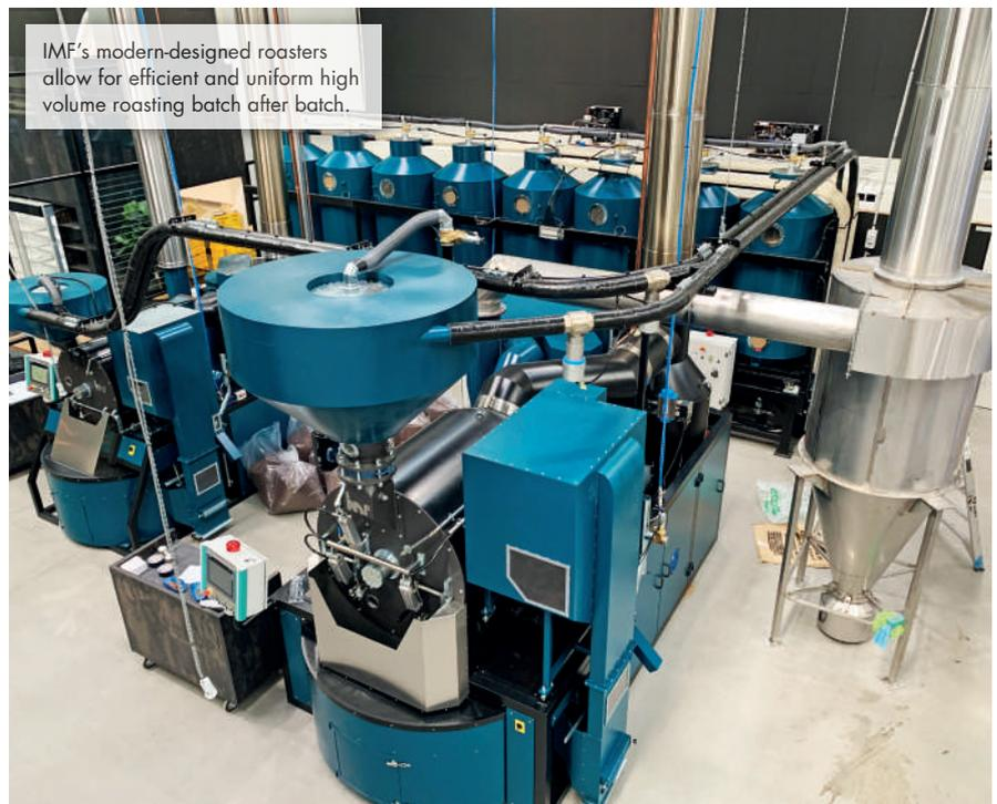
inside and surrounding the drum surface enters the roaster. This creates even heat distribution across the surface of the coffee beans, resulting in coffee roasted with precision and consistency.
